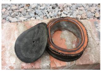
On checking the air filter, its mangled condition indicated one possible cause of the compressor malfunction.
