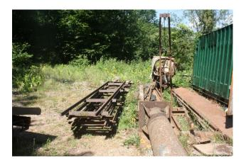
Traverser kit of parts at Lea Bailey awaiting laying out and installing on the mine tip.
