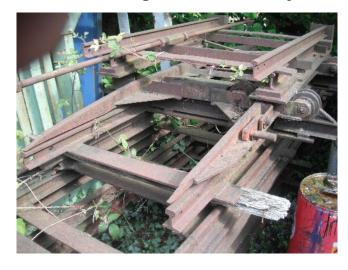
Recently bought from Alan Keef was a secondhand traverser. Seen here in Keefs yard awaiting delivery to Lea Bailey On top of the stack is the carriage, which runs on 2ft 6in gauge track (of which there is approx 20ft; also included is approx 40ft of 2ft gauge track).
