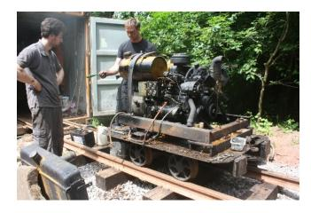
After the May open days it became apparent that the compressor in the mine tub was not delivering the expected 100 psi. It seemed to be overhesting and only delivering 40 psi. First stage fault-finding required removal of a side panel. But due to a misunderstanding all panels were removed.
