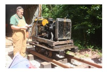
Unfortunately during removal of the panels the radiator was damaged so that now it leaks quite badly.
