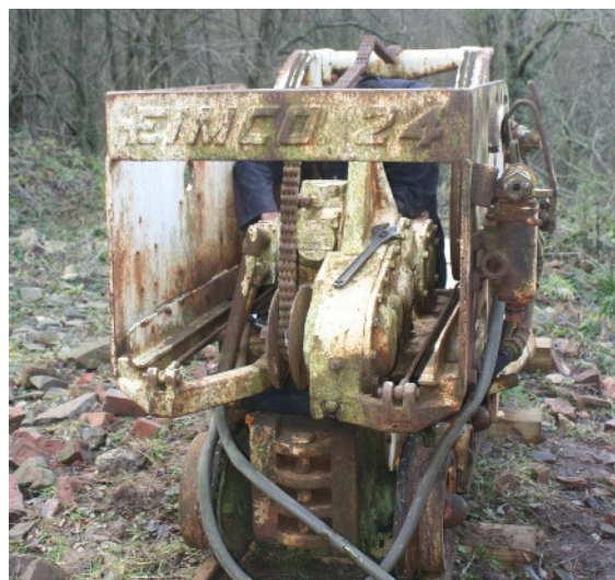
Photo:- Just visible is Nick loosening the bucket air motor retaining bolts.
