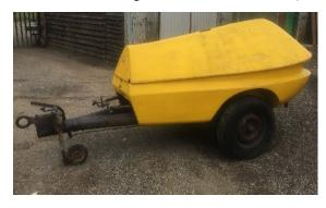
According to the Eimco operator's manual, our 12B rockershovel needs an air supply of 250 cfm (ft³/min), whereas a typical portable compressor (of the type available in the Forest) could only supply 150 cfm. The 70hp compressor with the supplementary air receiver should mean that we can operate the 12B, and a rockdrill as well as charging the 401 loco.
