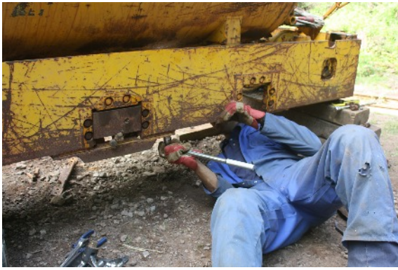
Then drop the axles and wheels after undoing axlebox bolts
