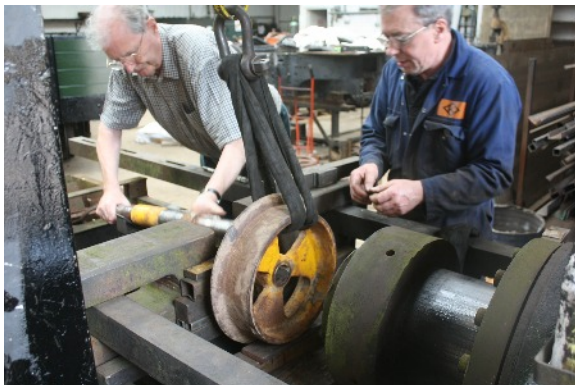
Ask Alan Keef to remove wheels and spacers and then refit, set to 2ft gauge
