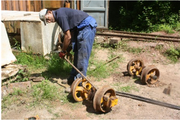
Remove axleboxes and old bearings from axles
