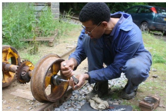
Fit new bearings to axles
