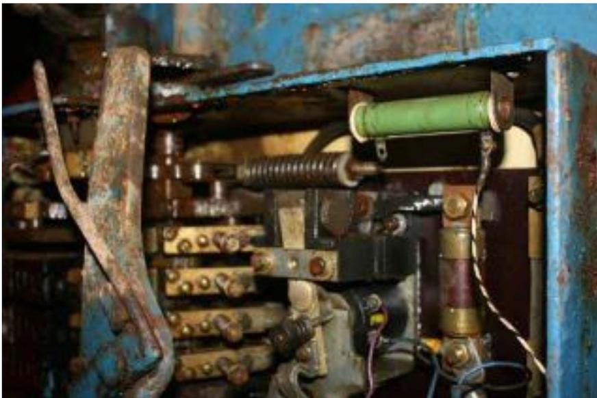
Work is proceeding well to get the Wingrove & Rogers battery electric loco running once more in the sheds at Clearwell. New cables and connectors are required to link four truck batteries. Donations are welcome for these, which will cost around £600
